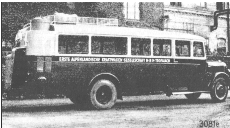
Illustration 1: A typical gaswagon which had originally been a conventional bus but which was subsequently retro-fitted with a gas-generator and a Saurer engine. 81
